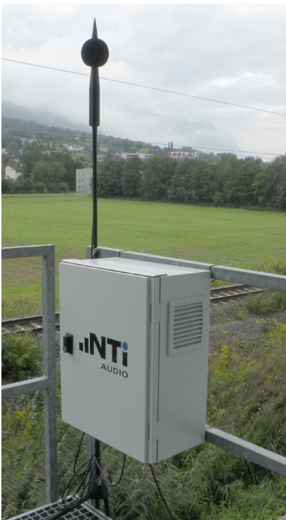
Noise Monitoring Terminal IP55 with outdoor mic mounted on tripod
