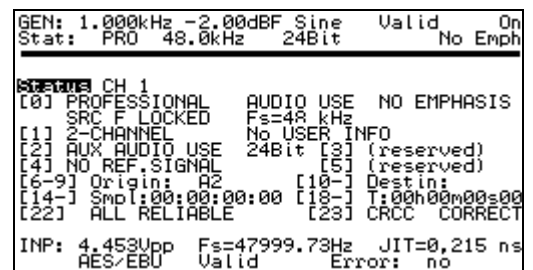
Fig 17 Channel Status in PRO Mode
