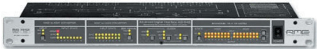
Figure: Example for a bi-directional, 64 channel ADAT to MADI Interface.
