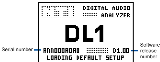
Fig 6-01, Start up screen loading default setup
