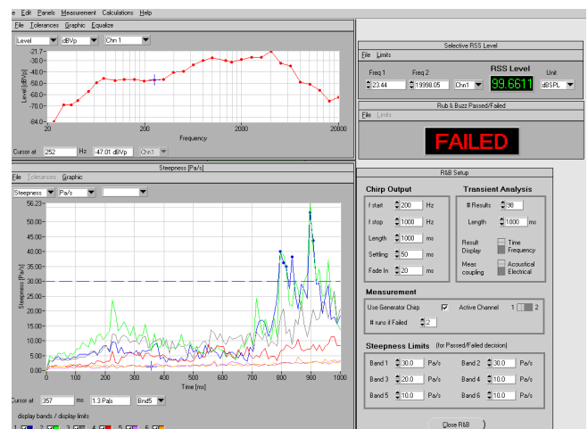
Figure 2: NTI Rub&Buzz test results - speaker with poor leadwire dress
