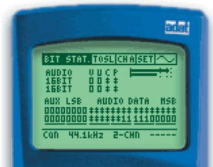
A/D converters sometimes show the problem that one digit of the output signal is not changing anymore. This is called 'bit stuck'. Such errors cause distortions of the converted audio signal. The DL1 measurement function 'Bit Statistics', immediately displays the audio resolution and any bits that continuously show '0' or '1'.
