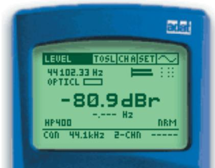
Internal converter defects or external mains power may cause distortion included in the digital audio signal. The Digilyzer enables the detection of such tricky faults. Just select the 'Level RMS' mode and read the displayed measurement value. Any DC offset or hum problems can be cut off by selecting the 'HP400' filter. So any change in the measurement value (with and without filtering) indicates the reported problem.
