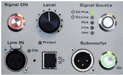
Control panel of PA3 Power Amplifier
