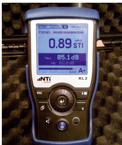
▲ Picture 2: Measurement of speech intelligibility with NTi Audio XL2
