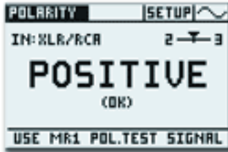
Polarity measurement function. XLR/RCA input must be selected from the input selector (IN).
