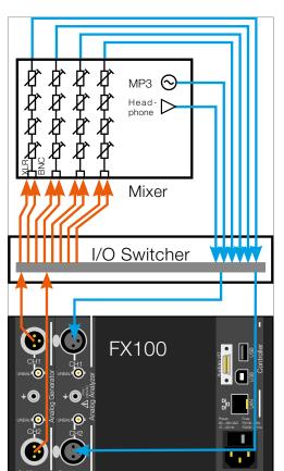
The new test setup successfully reduced the overall cycle time from approximately 30 minutes down to 6 minutes per mixing console.
