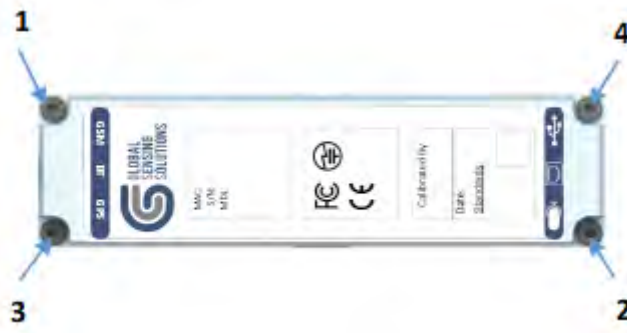
Figure 5 – Top Case Screw Removal Sequence
