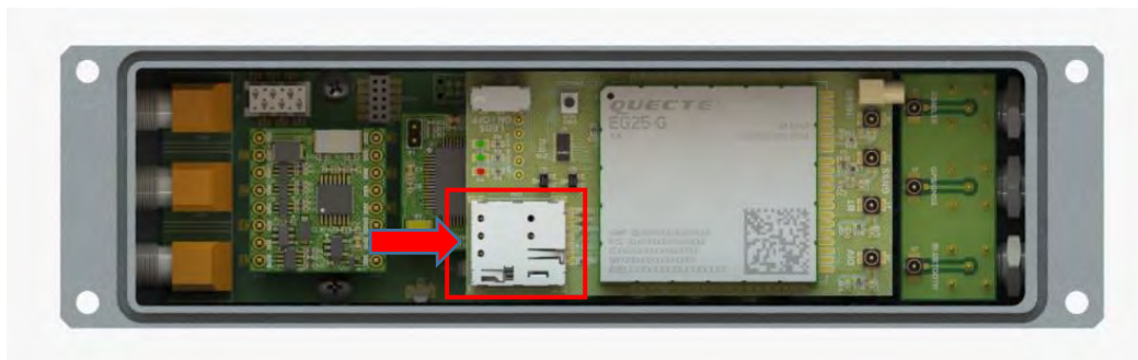
Figure 6 – Insert Nano SIM card
