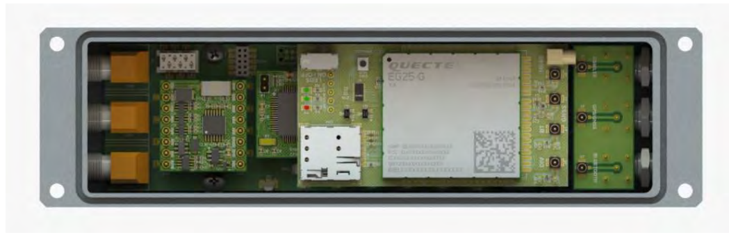
Figure 3 – 5GV Top Case inside view (communication module installed)
