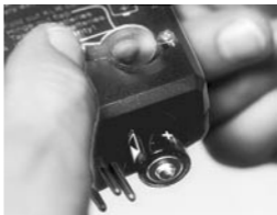
Fig 1 Insertion of batteries
