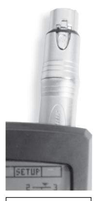
Thank you for buying the Adapter -20dB! This device extends the XLR input range of your Minilyzer or Acoustilyzer up to +40dBu.
