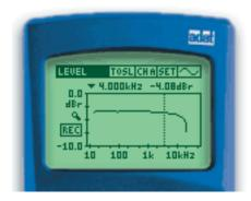
Use the Minirator MR1 as a signal source, select 'Sweep' and measure the frequency response at the A/D converter output with the DL1 in the 'Level RMS Sweep' mode. The result has to be a flat graph +/- 0.1 dB.
