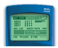
A/D converters sometimes show the problem that one digit of the output signal is not changing anymore. This is called 'bit stuck'. Such errors cause distortions of the converted audio signal. The DL1 measurement function 'Bit Statistics', immediately displays the audio resolution and any bits that continuously show '0' or '1'.
