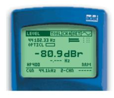
Internal converter defects or external mains power may cause distortion included in the digital audio signal. The Digilyzer enables the detection of such tricky faults. Just select the 'Level RMS' mode and read the displayed measurement value. Any DC offset or hum problems can be cut off by selecting the 'HP400' filter. So any change in the measurement value (with and without filtering) indicates the reported problem.
