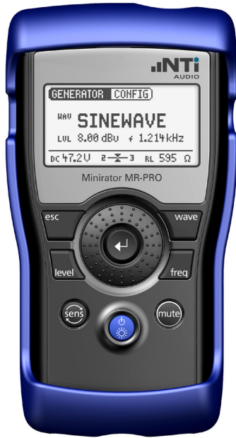
Minirator MR-PRO measures phantom power
