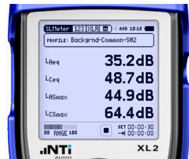
Background Noise Measurement by XL2 Sound Level Meter
