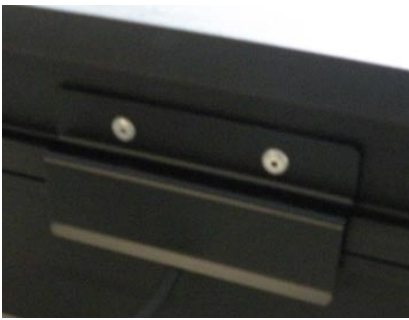
Rain-protected cable aperture with case closed (IP43 configuration)
