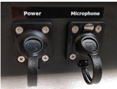
Waterproof connectors for microphone and external power supply (IP63 configuration)
