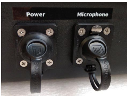
Waterproof connectors for microphone and external power supply (IP65 configuration)
