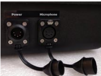
Removed protection plugs of waterproof connectors for microphone (IP65 configuration)
