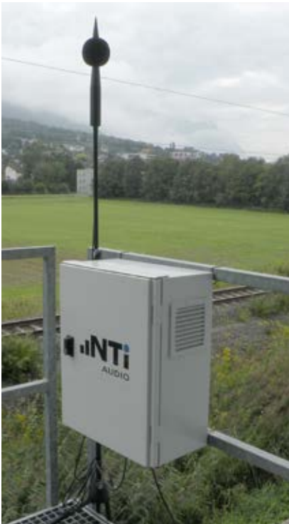
Noise Monitoring Terminal with outdoor mic mounted on tripod
