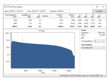
Calculate the FFT based on a recorded audio file for an objective audible assessment of tones in noise in accordance with the engineering methods described in ISO 1996:2-2017, DIN 45681 and BS 4142:2014.
