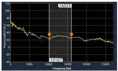
The microphone data obtained by the microphone array can be shown on the screen for a specific frequency bandwidth. When the spectrum is visible in the display, the bandwidth can be selected by touching the orange dot and drag this dot to the preferred frequency. Execute this for the lower and higher frequency. You can also move the selected frequency band by touching it in the middle and drag it to the preferred area of the spectrum.
