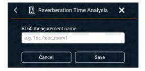
Create a project by entering the 'RT60 measurement name'. Tap on 'Save' to save the measurement or press 'Cancel' to stop.
