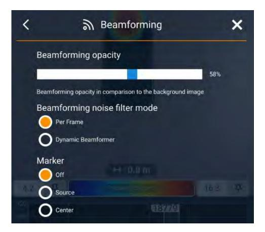
In addition, when the 'Dynamic Beamformer' is selected, the measurement distance will automatically adjust to the source location. If the 'Per Frame' is selected, the measuring distance needs to be adjusted manually in the home screen.
