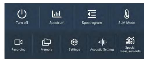
You can easily gain access to the different features and settings of the device. The required feature or setting can be selected by touching the related icon on the device. When the icon is selected it will turn orange (upper row) or white (bottom row). You can touch the icon again or press the "X" to close the feature or setting.
