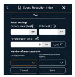
Enter the receiving room dimensions, the reverberation time of the receiving room, the number of speaker positions and the number of measurements per speaker position. The reverberation time can be loaded when you have performed a reverberation time measurement beforehand. This can be done by tapping the 'Load RT' button. Click on 'Save' once done.
