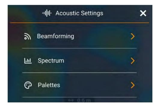
**Beamforming** Select 'Beamforming' to adjust the 'Beamforming opacity', to choose the noise filter mode 'Per Frame' or 'Dynamic Beamformer' and to add a 'Marker' showing an indication of the dB level (which is unweighted) at the marker point.
