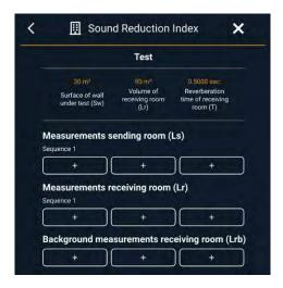
When one of the boxes is tapped, a button 'Start measurement' appears at the bottom. Click on 'Start measurement', and the 1/3 octave band values will be measured for 15 seconds and saved. After the measurement is finished, a checkmark appears on the box in place of +. If a measurement is already done, the user can redo the measurement if needed by tapping the box again.
