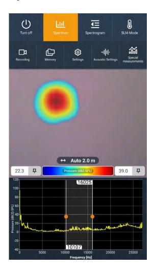
The microphone data obtained by the microphone array can be shown on the screen for a specific frequency bandwidth. When the spectrum is visible in the display, the bandwidth can be selected by touching the orange dot and drag this dot to the preferred frequency. Execute this for the lower and higher frequency. You can also move the selected frequency band by touching it in the middle and drag it to the preferred area of the spectrum.
