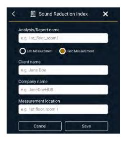
Create a project by entering the 'Analysis/Report name' and by choosing a measurement type. If 'Lab measurement' is chosen, the sound reduction index is denoted by R and if 'Field measurement' is chosen, the same index is denoted by R'. For further report purposes you can also input the 'Client name', the 'Company name' and the 'Measurement location'. Tap on 'Save' to save the measurement or press 'Cancel' to stop.
