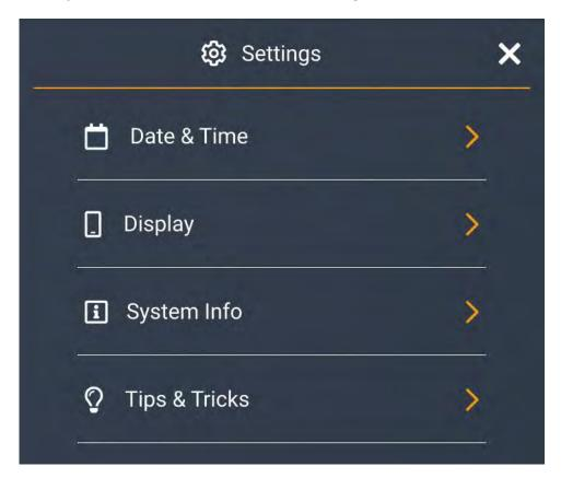
**Date & Time** Select 'Date & Time' to adjust the setting to 'Automatic' or 'Manual'. For the 'Automatic' setting you need a connection to the internet.
