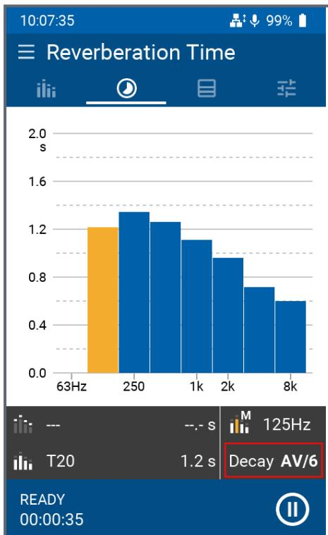
As soon as an initial measurement of the reverberation time has been performed, the device displays the spectral mean values. The single result of the yellow marked band appears below - you can select it with the arrow keys.
