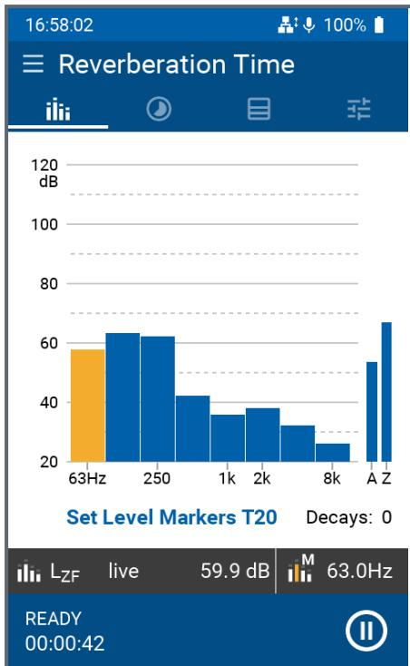
Here the spectrum of the current level is displayed in the selected resolution (octave or third octave bands).
