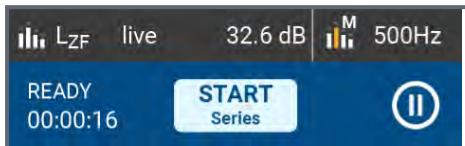
By tapping the **START Series** button, you start the measurement series and select the storage location.
