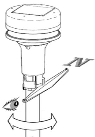
Note: Magnetic deviation must be considered to reference the measurements to True North.
