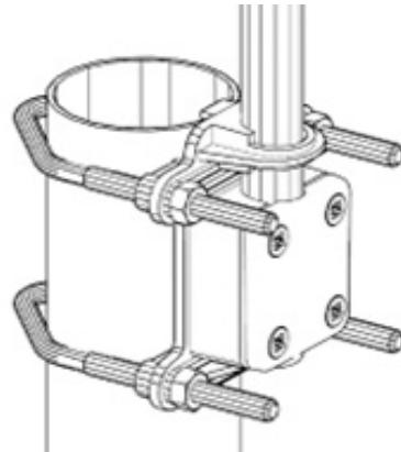
The sensor must be aligned to North. An alignment tool is supplied for this purpose. Clip the tool on the tube and slide it so that it snaps into the dedicated slots. Do not tamper with the slots. The tool must gently find its place. Slightly loosen the 4 screws that hold the tube. Align the tool - and the sensor - to North. Tighten the screws. Remove tools after use.
