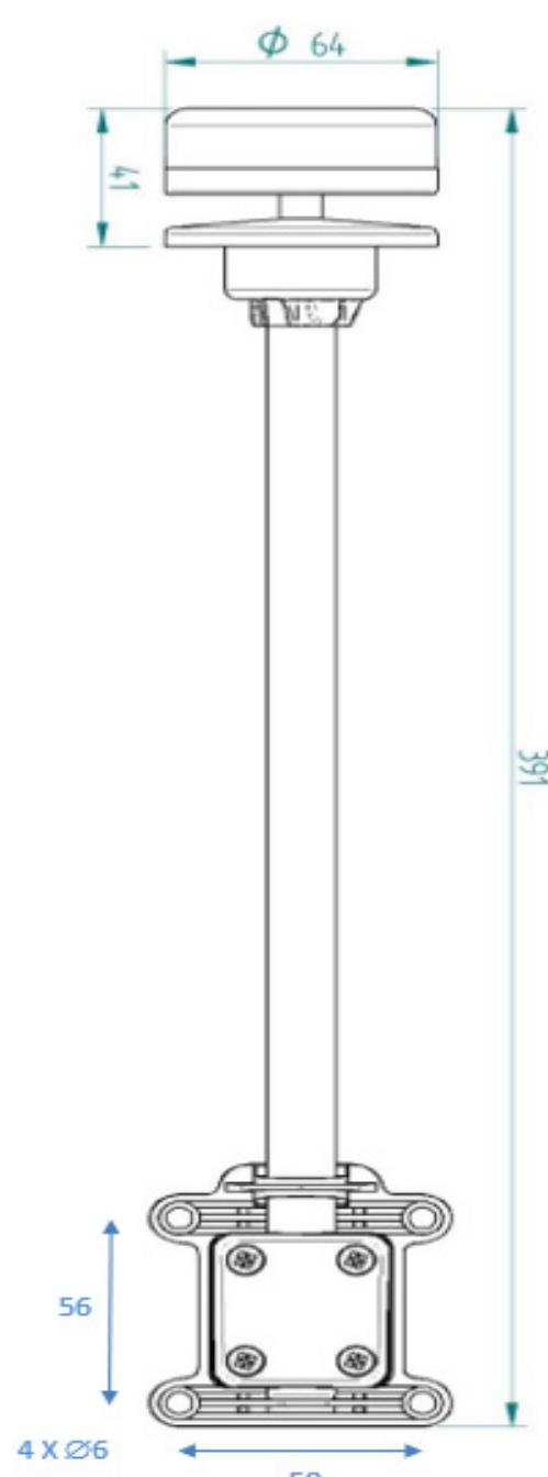
Sonic-Anemo-DLG-USB ultrasonic weather station is designed to be used with XL3 Acoustic Analyzer. Rugged design, no moving part and one single cable for the data transmission and power supply makes it robust and easy to use.
